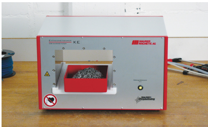
The parts are demagnetized by the demagnetizing pulse within mere seconds
