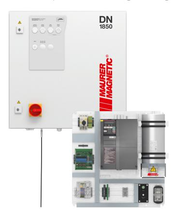
This power module includes the power, interface and control elements of the demagnetizing system. The connection cables between the coil module and the power module are pluggable. By default, the power module is configured in continuous mode; pulse operation is also available as an option.
