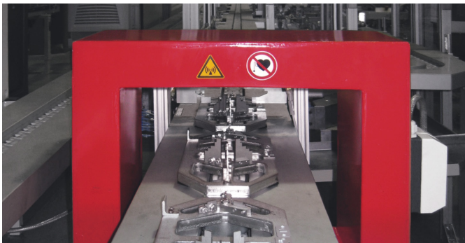
The coils even demagnetize reliably at maximum degrees of filling
